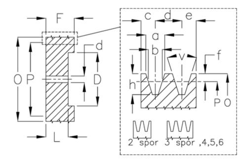
$\begin{array}{lll} D & = 97 \\ d & = 15 \\ F & = 80.0 \\ L & = 52 \\ Number of ribs = 5 \\ O & = 137.5 \\ P & = 132 \\ Type & = A \end{array}$
